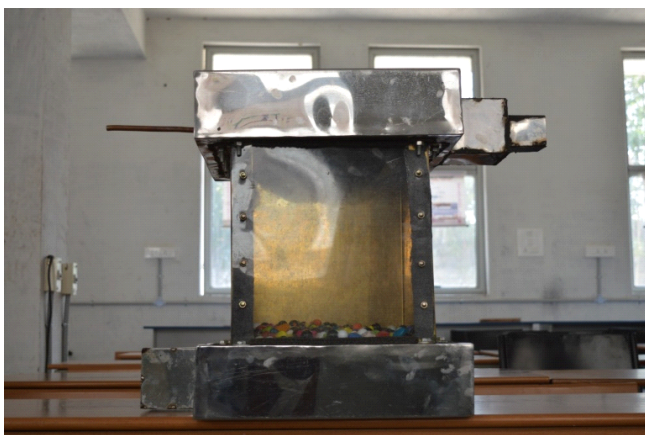
Fig. 2. Actual view of the specialized direct contact heat exchanger
