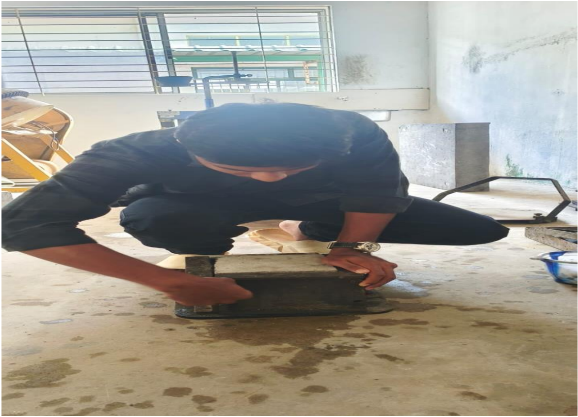
Fig 5 : Removal of Mould
